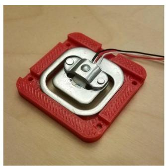
Figure 33. Load Cell Housing [3]
