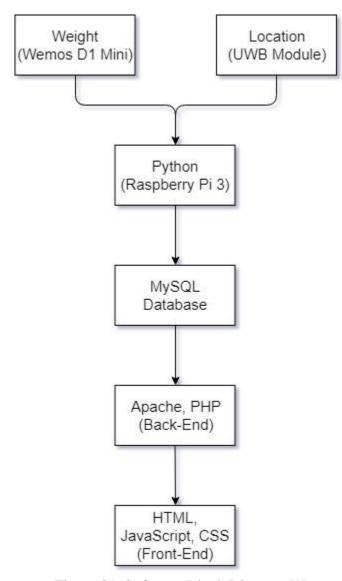
Figure 29. Software Block Diagram [9]
